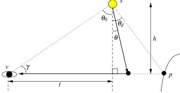
**Figure 3:** Diagram for angular reformulation of the airlight integral.
