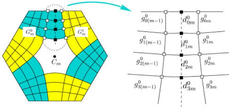
Fig. 12. Inserting the mid-edge point.
