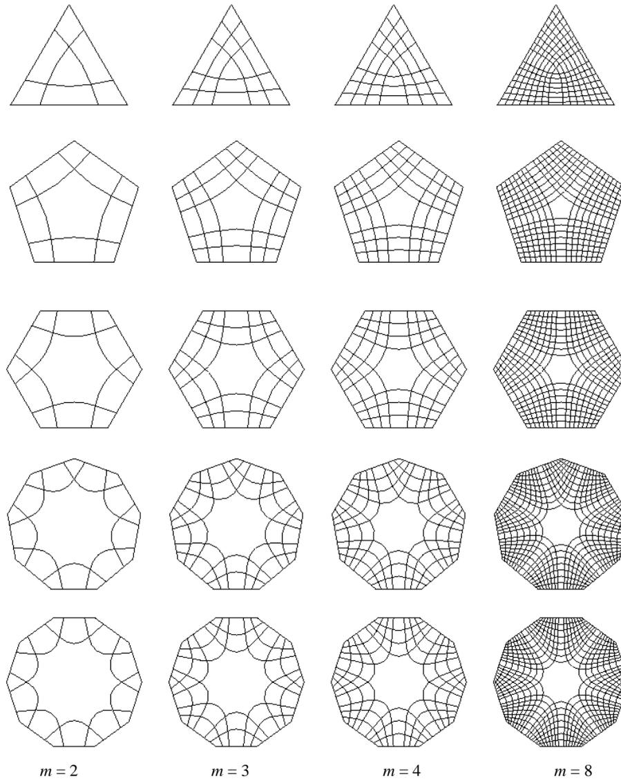
Fig. 4. Regular  $N$ -sided control meshes of different levels for  $N = 3, 5, 6, 9$ , and  $10$ .
