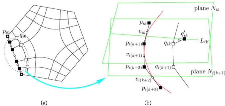
Fig. 8. The refinement of other interior vertices  $q_{ik}$  in step 2(a).
