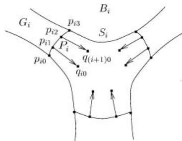
Fig. 10. Construction of a setback vertex blend.
