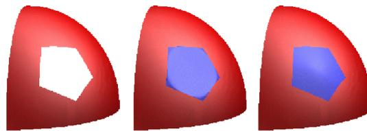
Fig. 15. Filling a 5-sided hole using fullness 0 (middle) and 1.0 (right).
