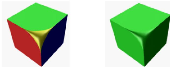
Fig. 18. A vertex blend of a box's corner having degenerated incident edge blends.
