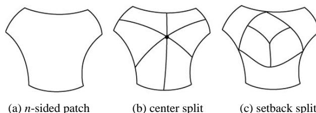
Fig. 2. Methods to construct the vertex blend.
