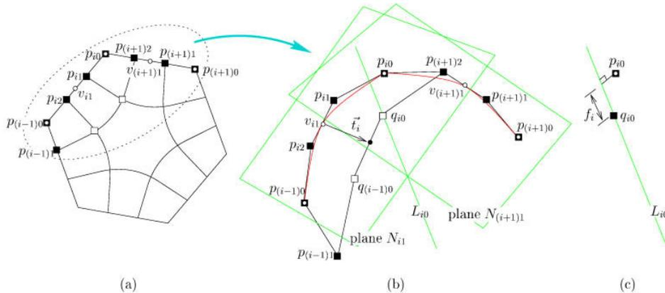
Fig. 6. The construction of an initial  $N$ -sided control mesh of level 3 in step 1.
