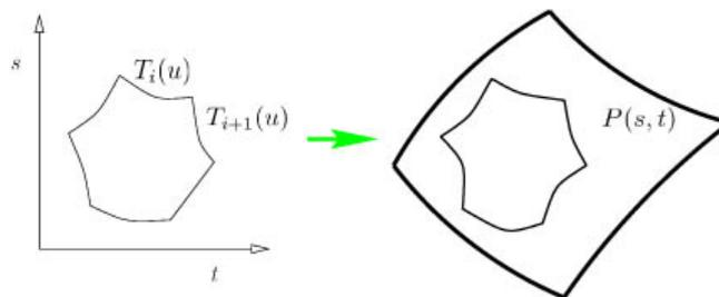
Fig. 5. An  $N$ -sided hole on a parametric surface.
