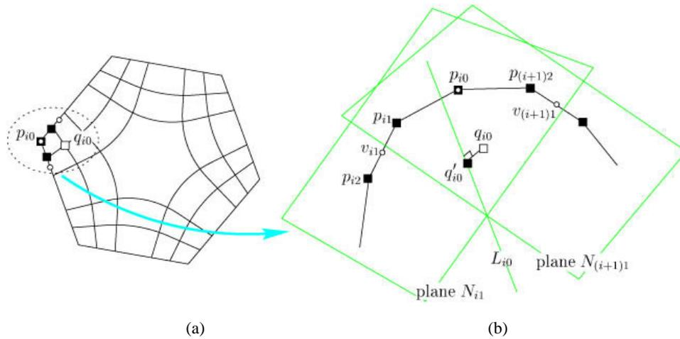
Fig. 7. The refinement of corner interior vertex  $q_{i0}$  in step 2(a).
